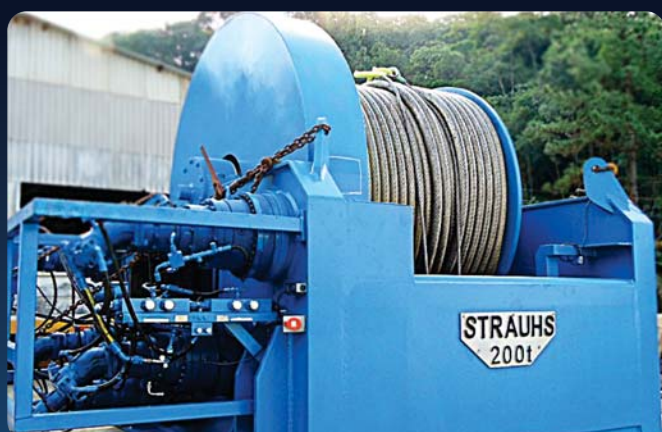
GUINCHO DE PULL-IN 200 TONS (5 MOTORES) – SYSTAC
